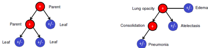
Fig.2 : A CNN was trained on a training set where all parent labels (red nodes) are positive, to classify leaf labels (blue nodes). For example, we train a CNN to classify Edema , Atelectasis , and Pneumonia on training examples where both Lung Opacity and Consolidation are positive.
